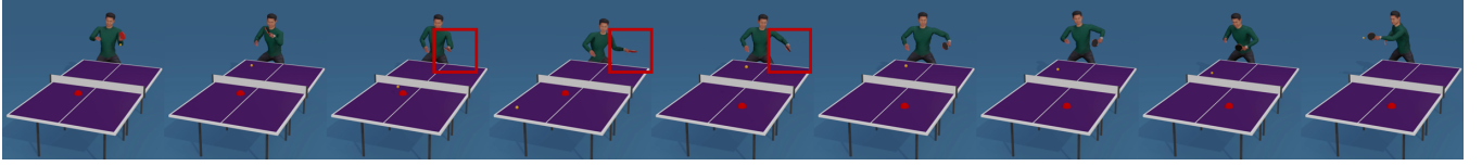
Figure 5: Transition results with only using forehand and backhand drive controllers. Both controllers are trained with random initialized configurations from the motion capture data. As shown in the red boxes, the agent attempts to use another forehand drive before the next ball is launched, which prevents it from switching back to a backhand drive in time.
