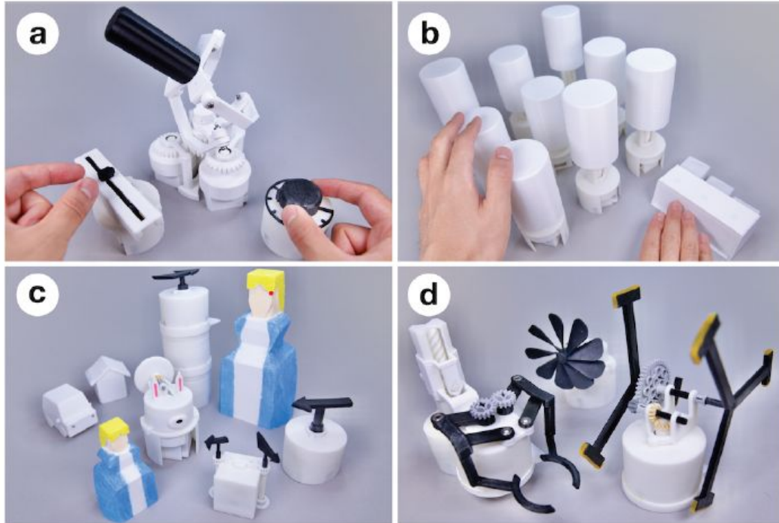
Figure 5-5: Overview of interaction design purposes and benefits of Mechanical Shells from instances of HERMITS (a. Tangible and Haptic Controllers, b. Data Physicalization / Tangible Representation, c. Storytelling with Expressive Shapes and Motion, and d. Extended Robotic Manipulator and Locomotion)
