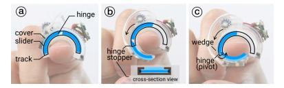
Figure 4: The key to our mechanism's unfolding is that (a) its cover is comprised of two segments; (b) our hinge is based on two detents that create a stopper and (c) force the cover to pivot and be pushed by the wedge against the fingerpad.
