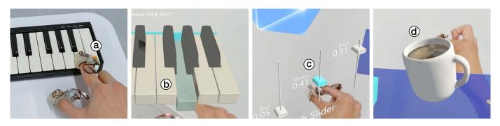
Figure 5: Adding contact haptic feedback to GUI widgets in existing Microsoft HoloLens Mixed Reality Toolkit (MRTK) while preserving the ability to feel physical objects: (a) pressing a physical piano key (b) pressing a virtual piano key (c) pinching a slider, (d) grabbing objects, a coffee mug in this case.
