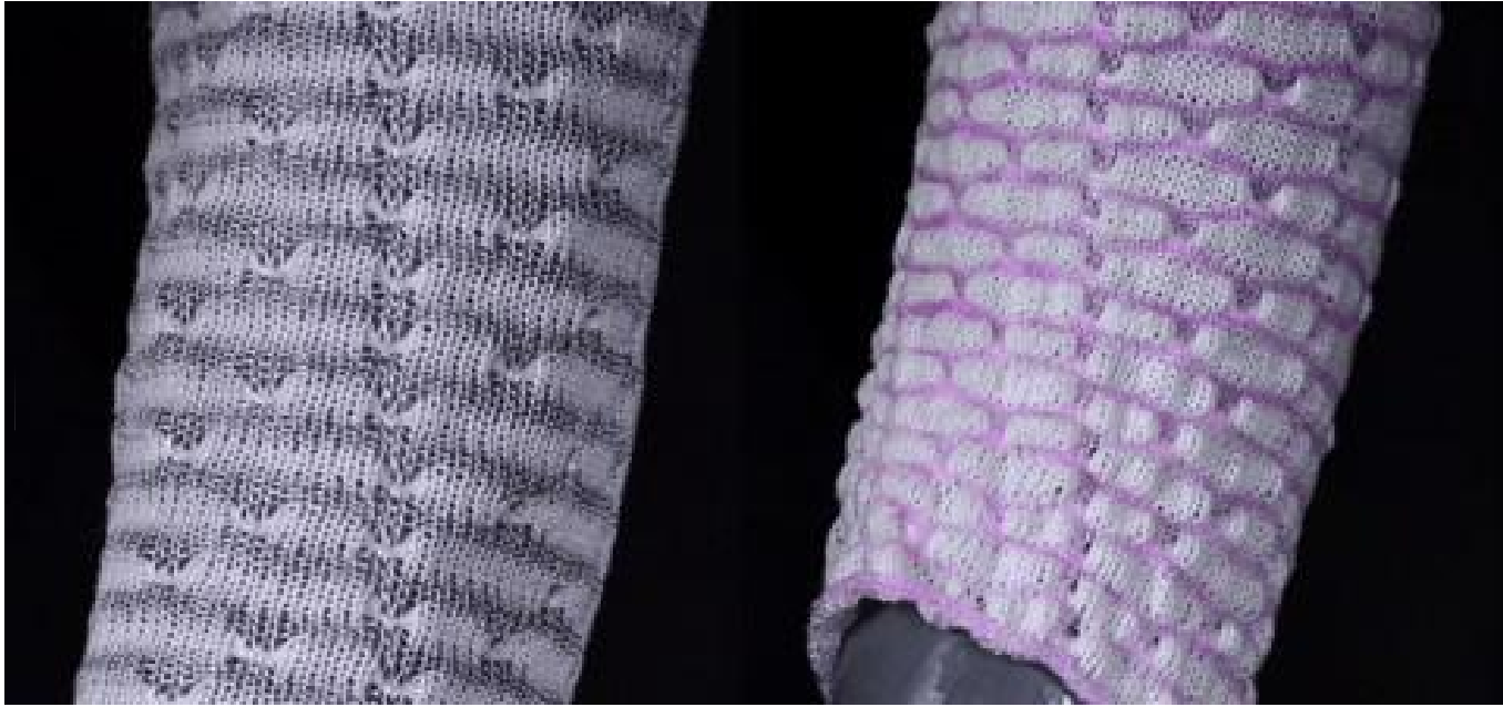
Figure 2: A textile sleeve shown before activation (Left) and after activation with porosity, shape and color change (Right).
