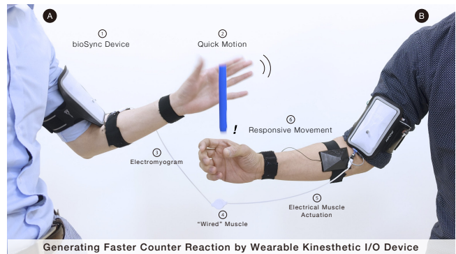
Figure 1: Wired Muscle: a system for directly connecting muscles of two persons. The EMG detects the muscle activity of a person A, which triggers the EMS to drive the muscle of person B to produce rapid corresponding movements.
